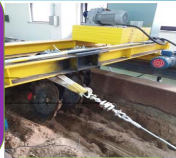
Draft Force measurement using a load cell
